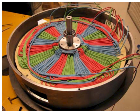
Figure 10: TVLM scale prototype. The upper rotor has been removed to show the stator windings.
