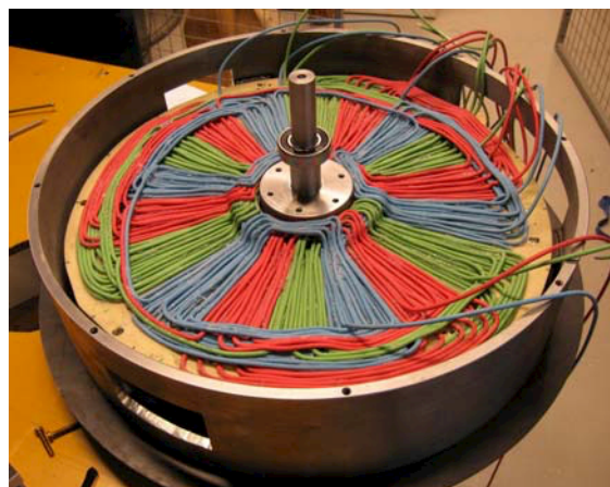
Figure 10: TVLM scale prototype. The upper rotor has been removed to show the stator windings.
