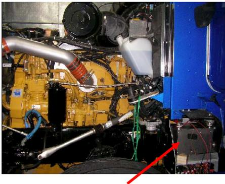
Figure 4: DLCAP module location in C-15 CAT diesel engine
