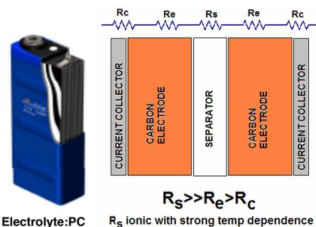
Figure 2: The basic elements forming the capacitor.
