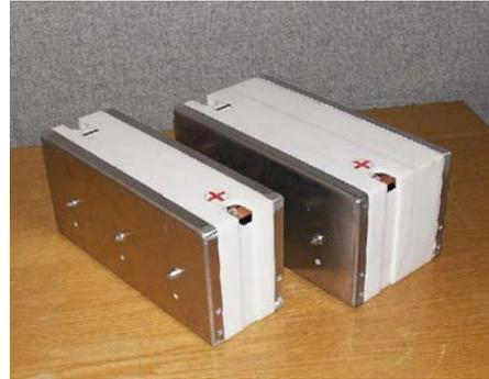
Figure 8: 3<sup>rd</sup> cranking, which exceeded 100 RPM at -30 °C with the initial capacitor module charged to 21V.
