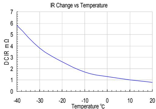
Figure 1: Temperature characteristic
