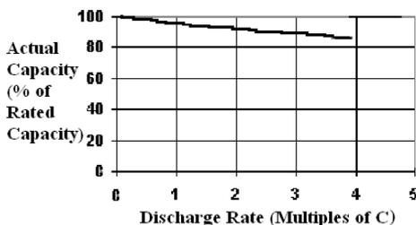
Figure 10: Effect of Discharge Rate on Capacity
