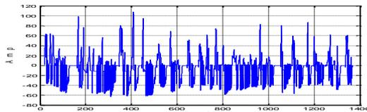
Figure 14: Battery current versus time for SOCmin=0.6 and SOCmax=1, over FTP 72 cycle.
