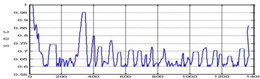
Figure 13: Battery SOC versus time for SOCmin=0.6 and SOCmax=1, over FTP 72 cycle.
