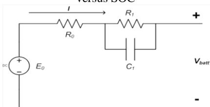
Figure 7: Randle first order battery electrical model.
