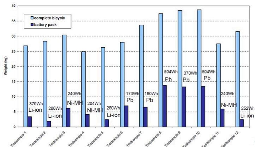
Figure 2: Weight information of the different test samples
