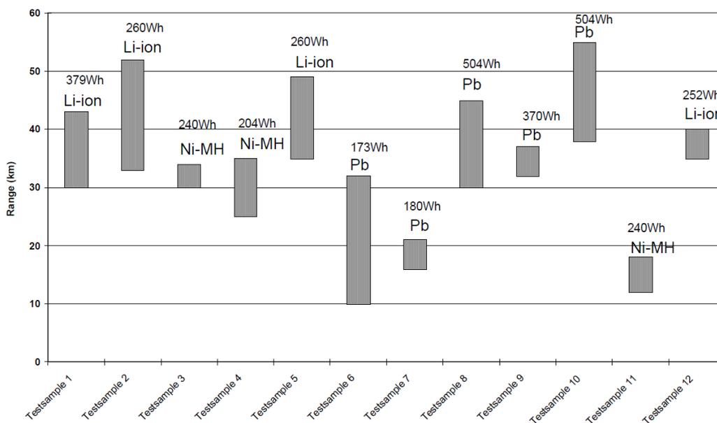
Figure 5: Spread of the driving ranges of the electric bicycles used in the highest assistance mode
