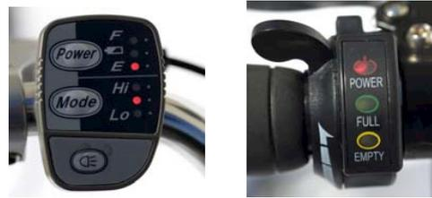
Figure 4: Selection of different assistance modes (left) and modulation of electrical assistance with a thumb switch (right)
