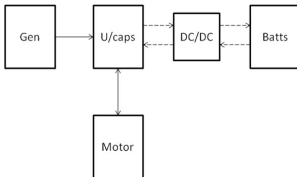
Figure 3 – Power flow in the DuoDrive system
