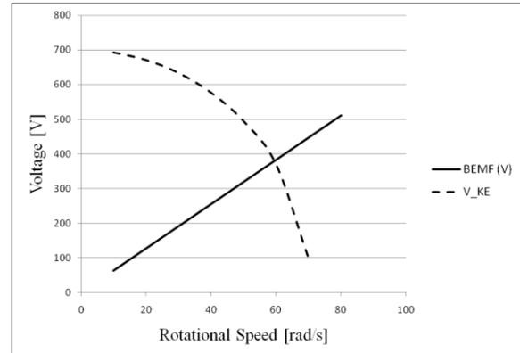
Figure 3 – DC Bus target voltage requirements
