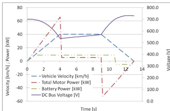
Figure 4 – Vehicle speed, ultracapacitor energy, battery power and motor power for Case1
