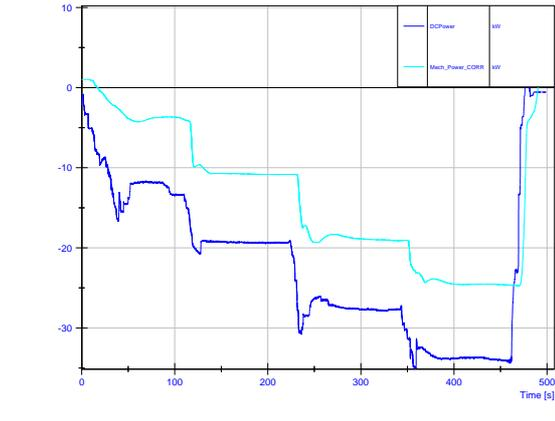
Figure 6: iOn electrical battery power (dark) and mechanical wheel power (light) at 80km/h test.
