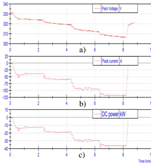
Figure 11: AGV measured a) battery voltage, b) battery current, c) resulting battery power, during 80km/h roller bench test.
