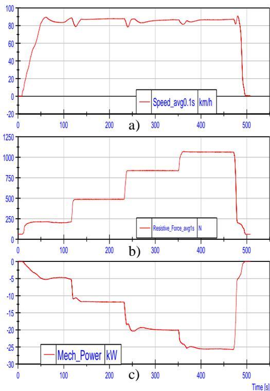
Figure 4: iOn measured a) speed, b) resistive force and c) (inversed) mechanical power at wheels during roller bench test at +/- 80km/h.
