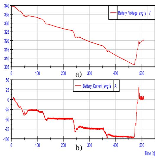
Figure 5: iOn measured a) battery voltage and b) battery current during +/-80km/h roller bench test.
